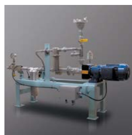
Aqueous urea spraying pump unit
