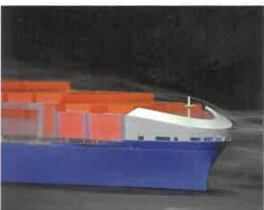
Ship Energy Saving Consultant: Containership Bow Wind-Shield
